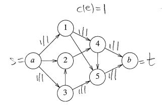
Show a flow network such that the solution to the maximum flow problem in this network will yield p(a,b). What is the value of p(a,b) in this case? p(a,b) = 2
