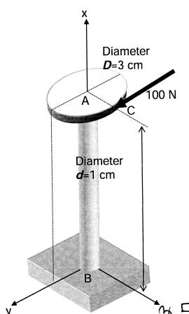
A force is applied at point C to a (very thin) circular **rigid** plate with diameter D=3cm. The plate is attached to an **elastic shaft** (AB) of diameter d=1cm and length L=10cm. All the strain energy is stored in the shaft (none in the plate since it is rigid). Also assume that strain energy stored due to transverse shear is negligible. The material is Aluminum (E=73 GPa, G=27 GPa)
