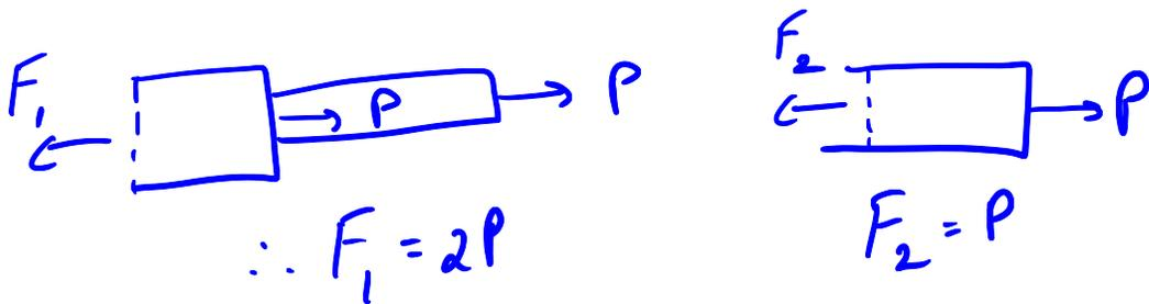
$$\begin{aligned} \text{a) } U_A &= \frac{1}{2} F_1^2 \left( \frac{L}{AE} \right)_1 + \frac{1}{2} F_2^2 \left( \frac{L}{AE} \right)_2 \\ &= \frac{1}{2} \left( \frac{L}{AE} \right) 5P^2 \end{aligned}$$
