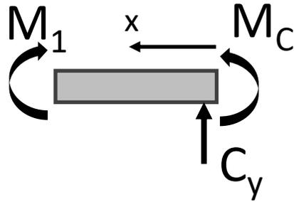
$$\left(\sum M\right)_1 = -M_1 + M_C + C_y x = 0 \quad M_1 = M_C + C_y x \quad (2)$$
