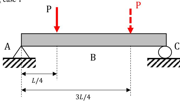
Considering the symmetry, the Force  $P$  at  $x = L/4$  (solid line) and  $P$  at  $x = 3L/4$  (dashed line) will produce the same deflection for the roller B. Thus,
