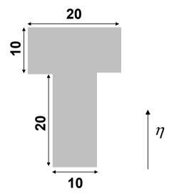
$$\frac{\text{Centroid:}}{\overline{\eta} = \frac{25(20 \times 10) + 10(20 \times 10)}{2(20 \times 10)} = 17.5 mm}$$
