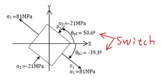
Having found the principal stress values and the orientation of the principal plane, a material element can be drawn as shown on the side.
