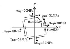
On the plane of maximum in-plane shear stress the normal stresses are the average normal stress given by  $\sigma_{avg}=\frac{\sigma_x+\sigma_y}{2}=\frac{20+40}{2}=30\,MPa$ . With this we can plot the material element for the maximum in-plane shear stress as shown on the side.
