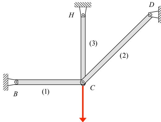
Consider the truss above that is made up of elements (1), (2) and (3).
