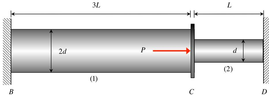
A rod is made up of solid elements (1) and (2) joined by a rigid connector C, with the material of (1) and (2) having the same modulus of elasticity  $E$ . An axial load  $P$  is applied to C with no thermal loads being present. Let  $F_1$  and  $F_2$  represent the axial loads in elements (1) and (2), respectively. Circle the response below which most accurately describes the relative sizes of  $|F_1|$  and  $|F_2|$ :
