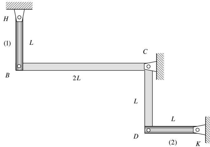
Identical elements (1) and (2) (each having a Young's modulus  $E$ , coefficient of thermal expansion  $\alpha$  and cross-sectional area  $A$ ) are connected between ends  $B$  and  $D$ , respectively, of a rigid, L-shaped bar  $BCD$ . The temperature of (1) is *increased* by an amount of  $\Delta T > 0$ , with the temperature of element (2) being held constant.
