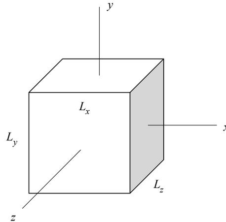
A cube of dimensions  $(L_x, L_y, L_z)$  experiences a state of stress with uniform components of stress throughout the cube. The material of the cube has a Young's modulus of  $E$  and a Poisson's ratio of  $\nu = 0.4$ . As a result of the loading on the cube, it is known that  $\sigma_y = \sigma_z = \sigma_x / 2 > 0$ . As a result of this loading (circle the correct answer):
