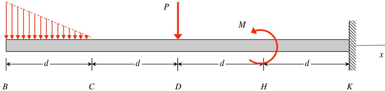
The above loading is applied to a cantilevered beam. *Circle* the figure below which most accurately describes the internal shear force resultant in the beam between locations B and C.
