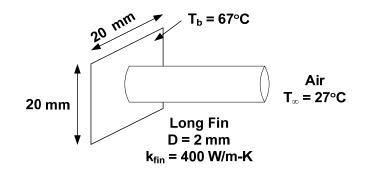
(a) Calculate the average convective heat transfer coefficient  $(W/m^2-K)$  on the fin surface. Since the surface temperature varies, you can use a representative fin surface temperature equal to the average of the base and tip temperatures in this calculation.
