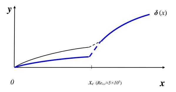
In the laminar region, the velocity and thermal boundary layer thicknesses have the relation of  $\frac{\delta}{\delta_t} \approx Pr^n$ , where  $n \approx \frac{1}{3}$ . For turbulence, the severe mixing leads to  $\delta_t \approx \delta$ .
