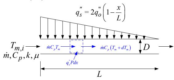
(a) (4 pts) Using an appropriate correlation, write an expression for convective heat transfer coefficient *h* inside the tube only in terms of known parameters.
