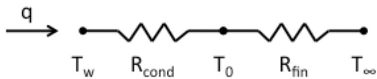
$$R_{cond} = \frac{L_1}{k \cdot A_c} = \frac{L_1}{k \cdot \frac{\pi D^2}{4}} = \frac{(0.2 \text{ m})}{(100 \text{ W/m-K}) \cdot \frac{\pi (0.025 \text{ m})^2}{4}} = 4.07 \text{ K/W}$$
